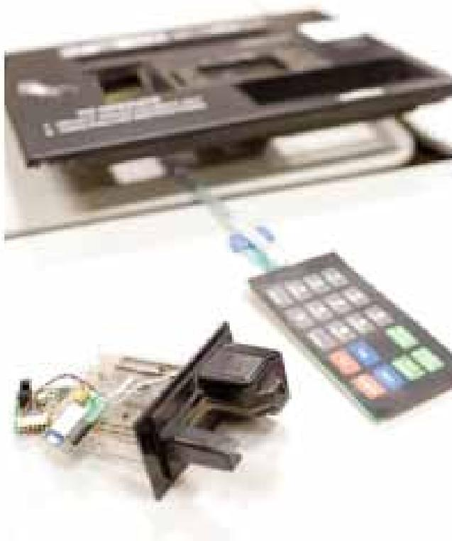
*Once a criminal has access, investigators familiar with this type of attack report that it only takes crooks about 30 seconds to remove the entire card device from a gas pump and replace it with an identical one fitted with electronic skimmers.*
